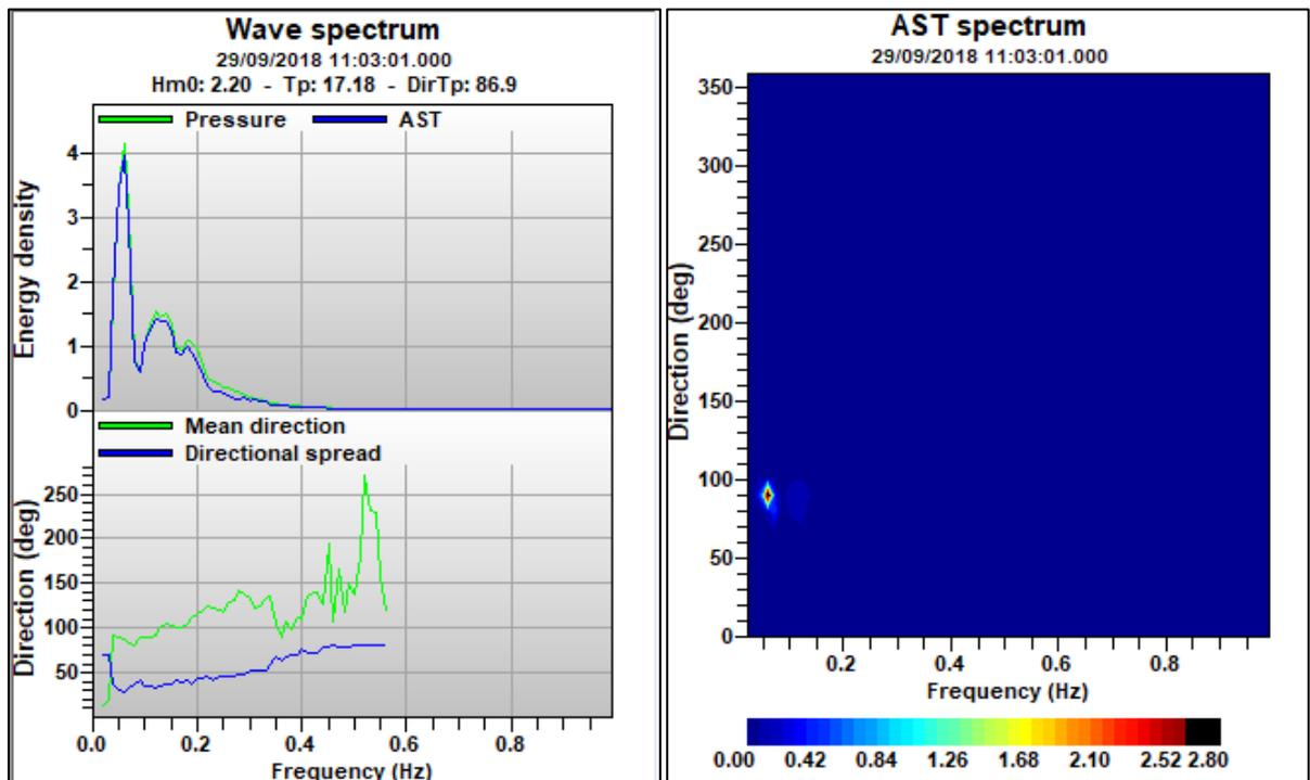
**Figure 7b: Processed wave data from STORM software**
