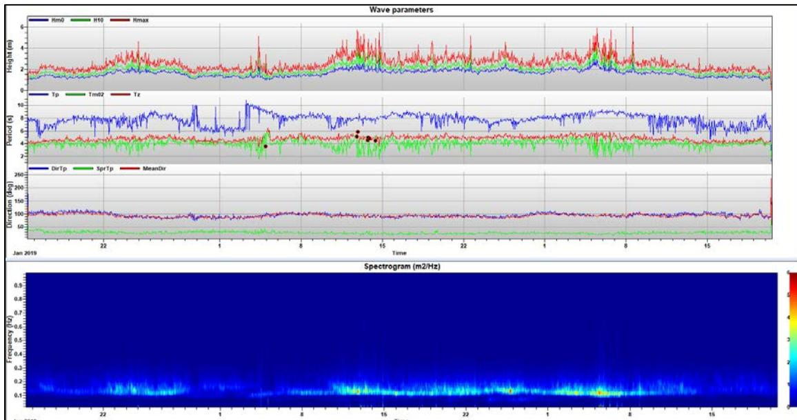
Figure 11a: Processed wave data from STORM software
