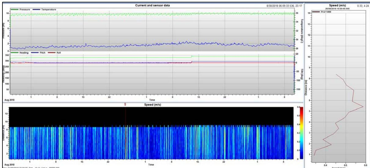
**Figure 6: Processed current data from STORM software**
